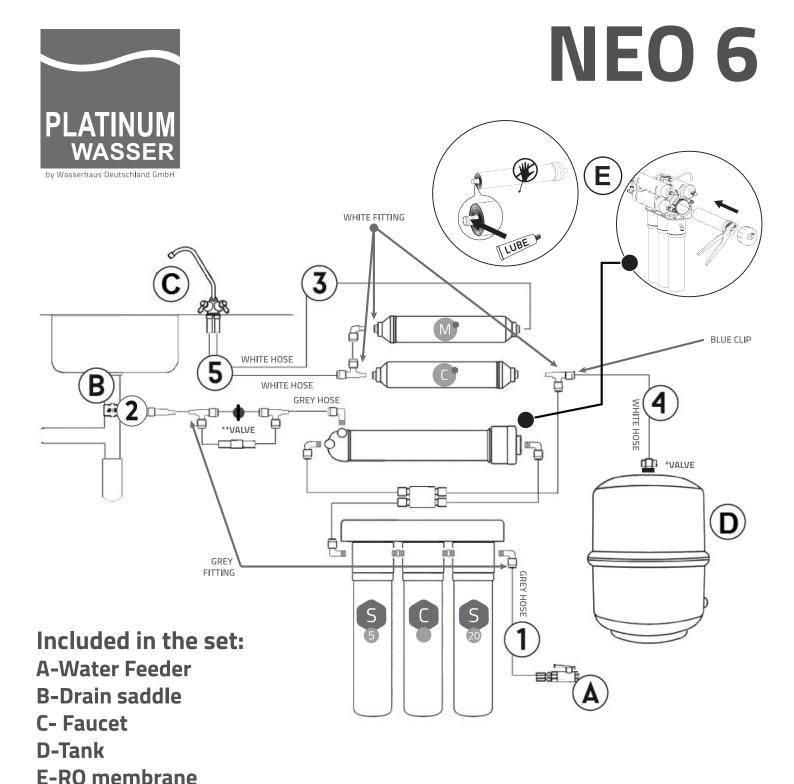
Parts of the filter inside the box are disconnected in places labelled with numbers 12345
