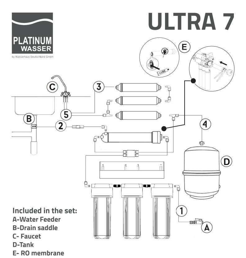
Parts of the filter inside the box are disconnected in places labelled with numbers 1,2,3,4,5. Please assemble the filter by using a 1/4" tube.
